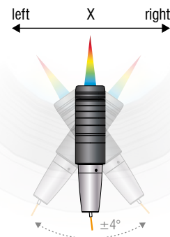
3 Max. tilt angle in X \pm 4^\circ
