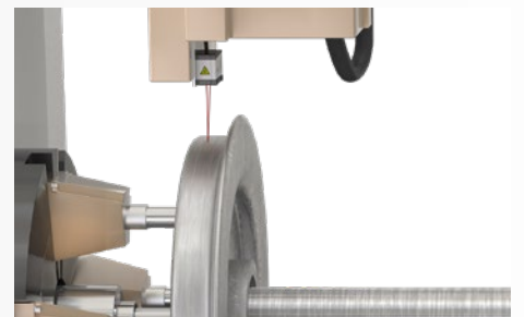
Wear inspection of wheel tires
