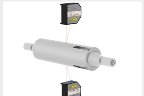
Testing the radial run out of rollers
