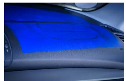
Full-surface back projection of the inspection result
